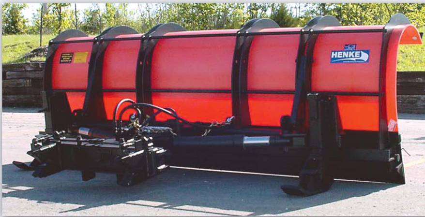
▲ Henke 43R11J Poly Shown with Optional Runners and Quick Hitch
